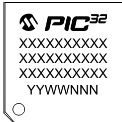
64-Lead TQFP (10x10x1 mm)
