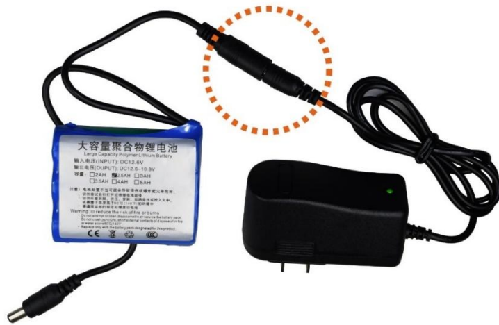
Figure 6-2 Connect charger to battery connector
