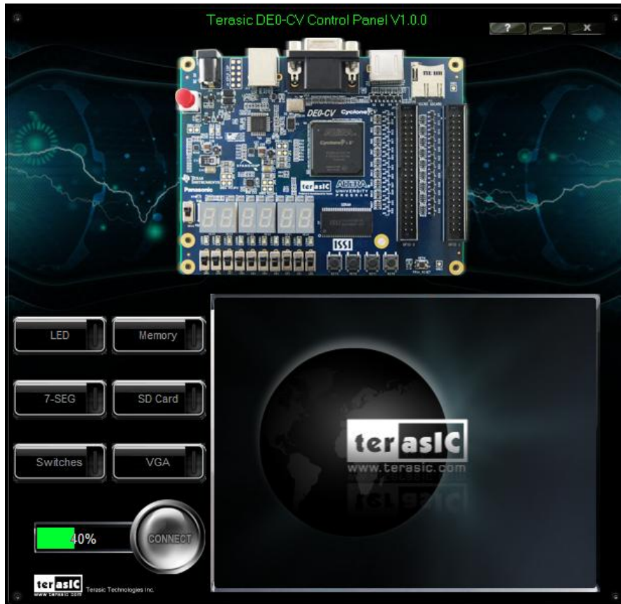
Figure 2-1 The DE0-CV Control Panel
