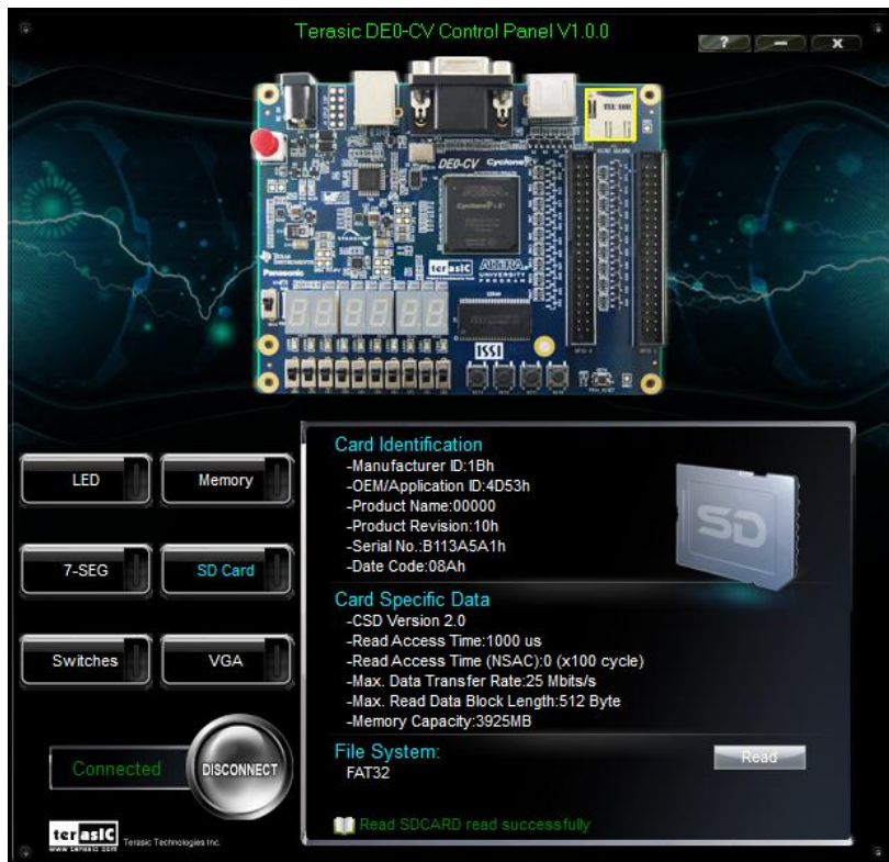
Figure 2-7 Reading the SD Card Identification and Specification
