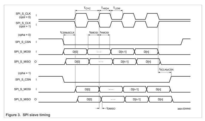
Write operations of NXH3670UK SPI slave interface can be done with a clock frequency of 16 MHz. However, for read operations in the final application, the MISO output delay can impact the performances.
