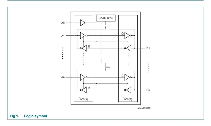
2-bit dual supply translating transceiver; open drain; auto direction sensing
