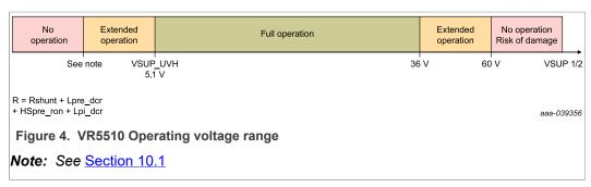
Below the VSUP\_UVH threshold, the extended operation range depends on the VPRE output voltage configuration and the external components.
