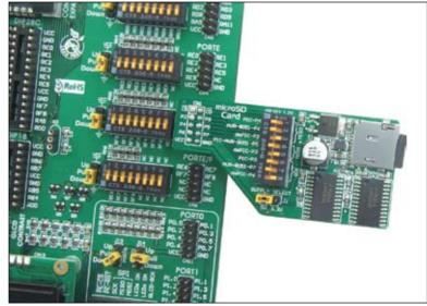
Figure 4: microSD Card connected to a development system
