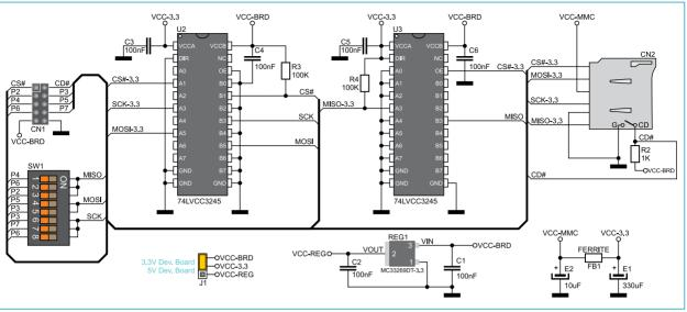
Figure 3: microSD Card additional board connection schematic
