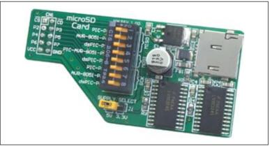
Figure 1: microSD Card additional board
