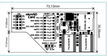
Figure 2: Dimensions of the microSD Card additional board
