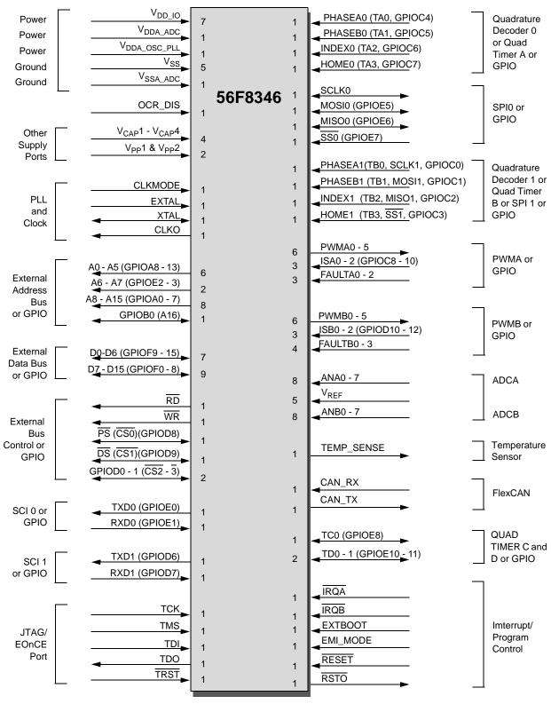
Figure 2-1 56F8346 Signals Identified by Functional Group<sup>1</sup> (144-pin LQFP)
