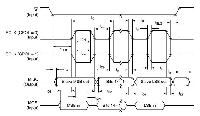
Figure 10-12 SPI Slave Timing (CPHA = 0)
