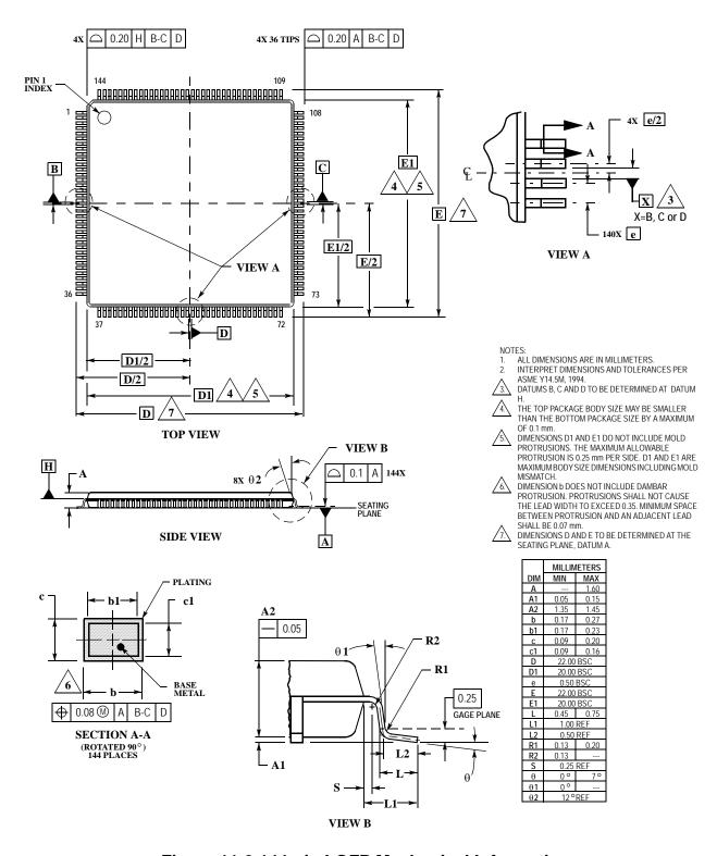
Figure 11-3 144-pin LQFP Mechanical Information
