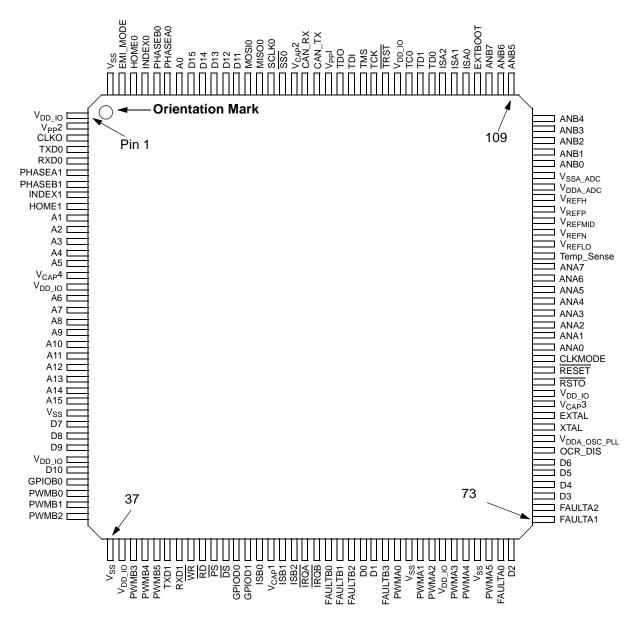
Figure 11-1 Top View, 56F8346 144-Pin LQFP Package
