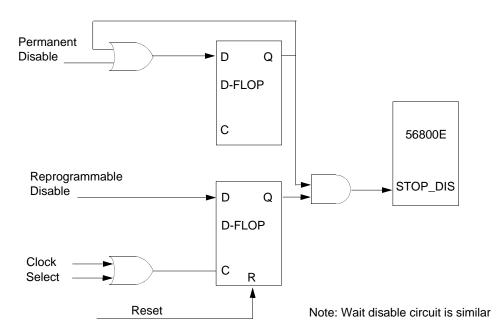
Figure 6-16 Internal Stop Disable Circuit
