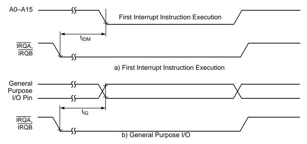
Figure 10-7 External Level-Sensitive Interrupt Timing
