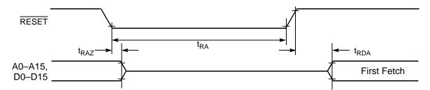
**Figure 10-5 Asynchronous Reset Timing**
