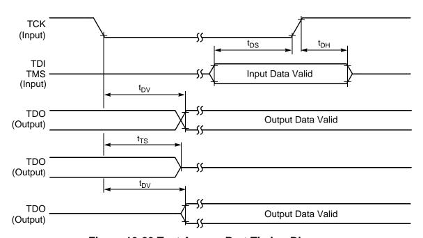
Figure 10-20 Test Access Port Timing Diagram
