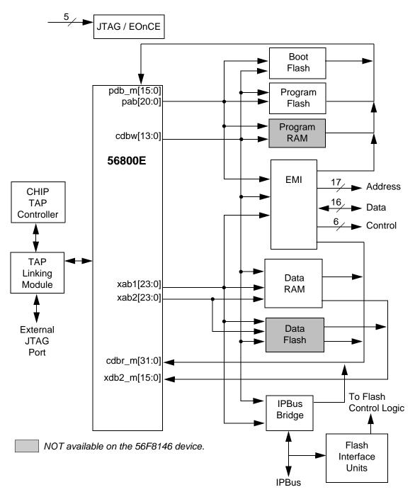
Figure 1-1 System Bus Interfaces
