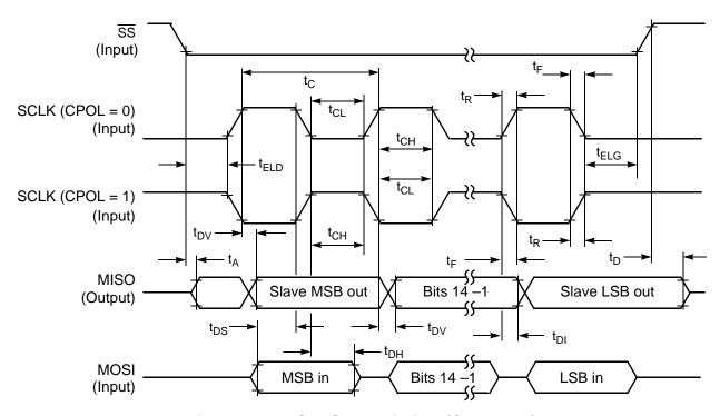
Figure 10-13 SPI Slave Timing (CPHA = 1)
