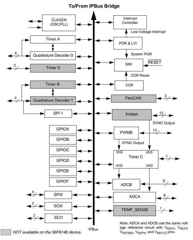
Figure 1-2 Peripheral Subsystem
