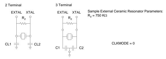
Figure 3-3 Connecting a Ceramic Resonator
