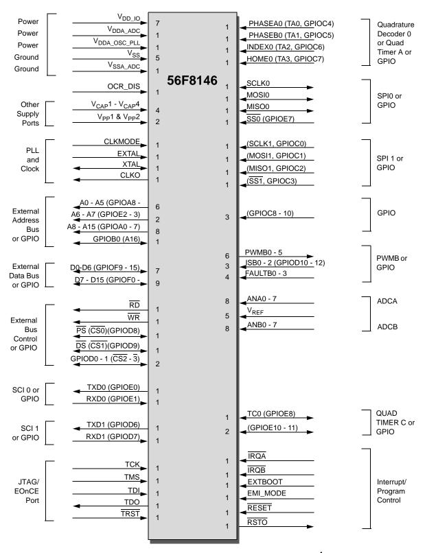
Figure 2-2 56F8146 Signals Identified by Functional Group<sup>1</sup> (144-pin LQFP)
