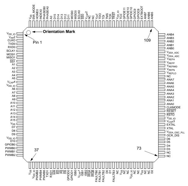
Figure 11-2 Top View, 56F8146 144-Pin LQFP Package
