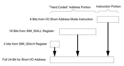
Figure 6-13 I/O Short Address Determination
