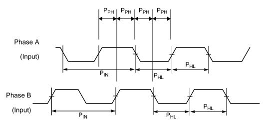
Figure 10-15 Quadrature Decoder Timing
