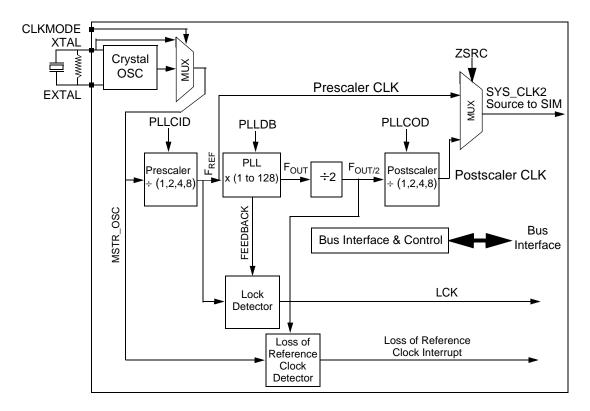
Figure 3-1 OCCS Block Diagram
