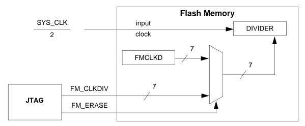
Figure 7-1 JTAG to FM Connection for Lockout Recovery
