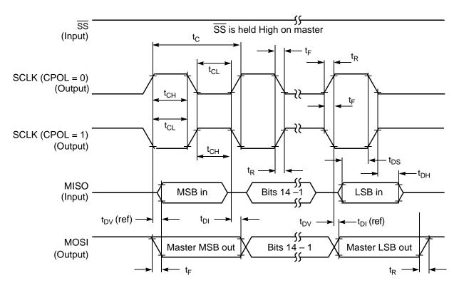
Figure 10-11 SPI Master Timing (CPHA = 1)
