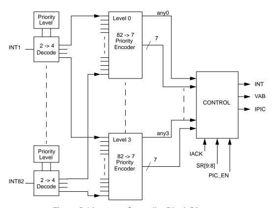
Figure 5-1 Interrupt Controller Block Diagram
