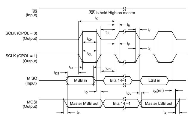
Figure 10-10 SPI Master Timing (CPHA = 0)
