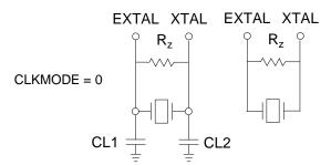
Sample External Crystal Parameters:  $R_z = 750 \text{ K}\Omega$
