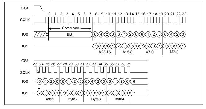
Figure 12. Dual I/O Fast Read Sequence Diagram ((M5-4) ≠ (1, 0))
