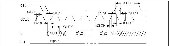
Figure 40. Output Timing
