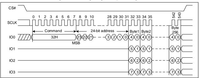
Figure 18. Quad Page Program Sequence Diagram
