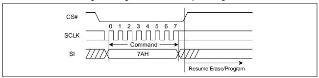
Figure 31. Program/Erase Resume Sequence Diagram
