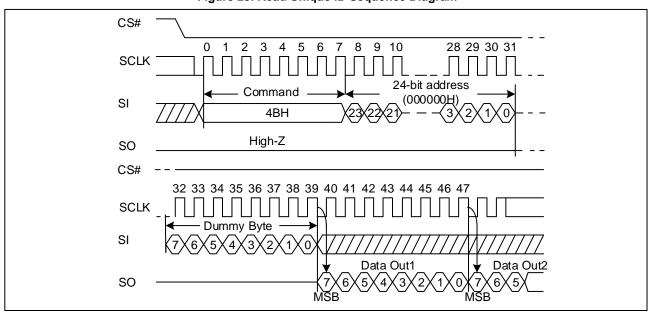
Figure 25. Read Unique ID Sequence Diagram
