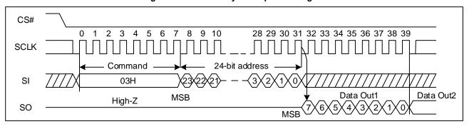
Figure 8. Read Data Bytes Sequence Diagram
