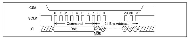
Figure 21. 64KB Block Erase Sequence Diagram
