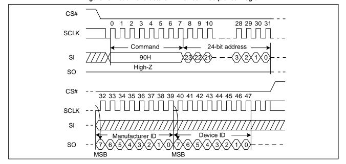
Figure 23. Read Manufacture ID/ Device ID Sequence Diagram
