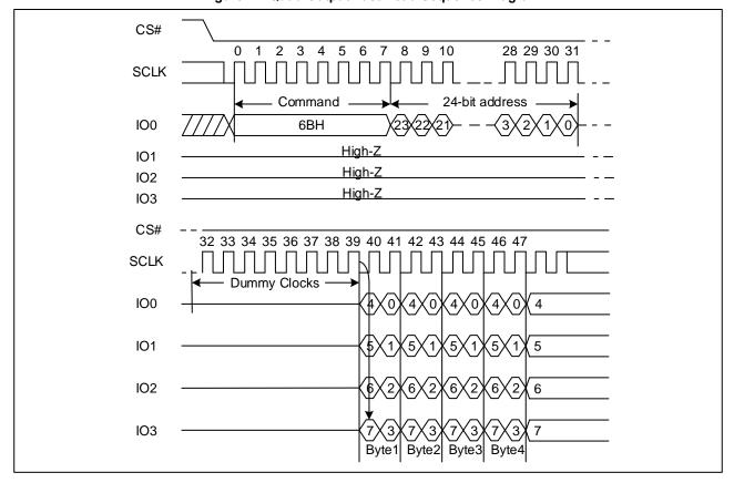
Figure 11. Quad Output Fast Read Sequence Diagram
