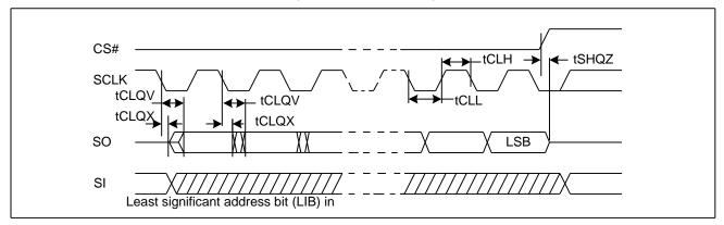
Figure 41. Resume to Suspend Timing Diagram
