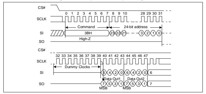
Figure 10. Dual Output Fast Read Sequence Diagram
