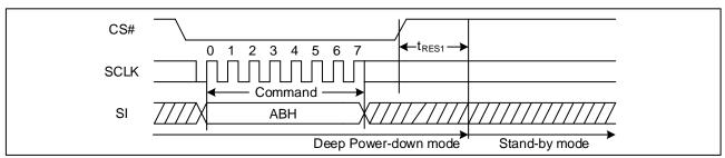
Figure 33. Release Power-Down Sequence Diagram
