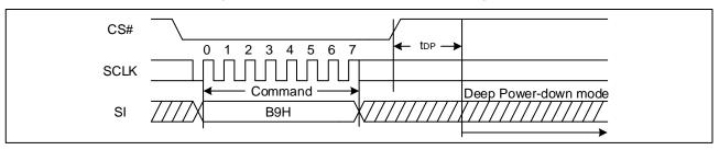
Figure 32. Deep Power-Down Sequence Diagram
