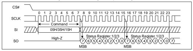
Figure 5. Read Status Register Sequence Diagram
