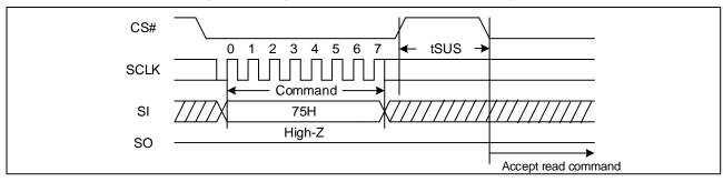
Figure 30. Program/Erase Suspend Sequence Diagram
