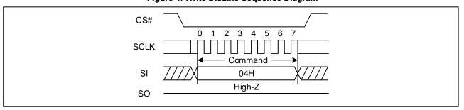
Figure 4. Write Disable Sequence Diagram
