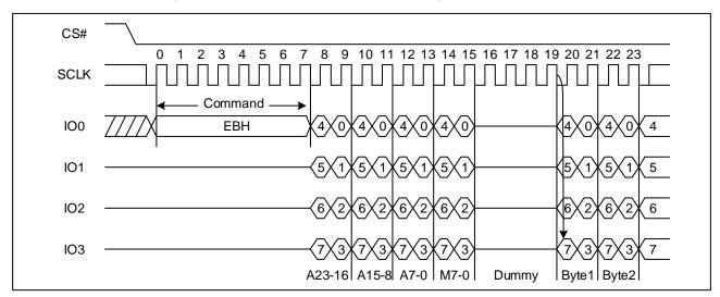
Figure 14. Quad I/O Fast Read Sequence Diagram ((M5-4) ≠ (1, 0))
