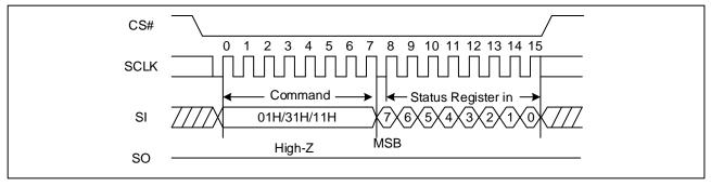
Figure 6. Write Status Register Sequence Diagram
