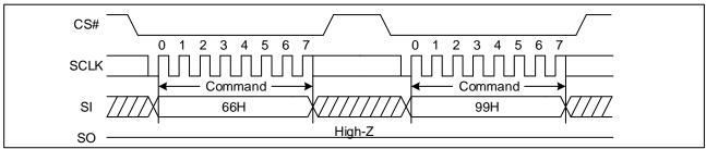
Figure 29. Enable Reset and Reset command Sequence Diagram
