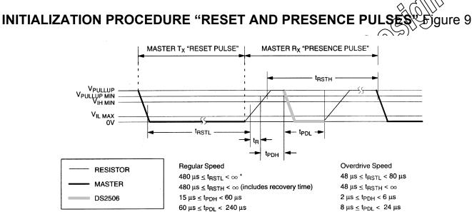
\* In order not to mask interrupt signalling by other devices on the 1-Wire bus,  $t_{RSTL} + t_R$  should always be less than 960 µs.
