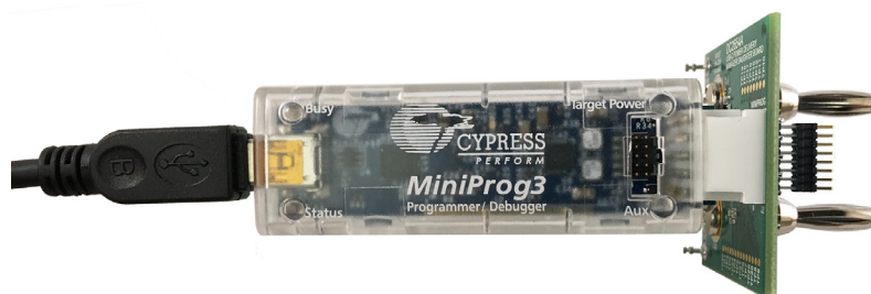
Figure 4. MiniProg3 Connected to DC2654A for Programming and Debugging
