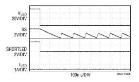
Short LED Protection with R<sub>SS</sub>: Latchoff Mode
