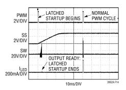
Figure 14. PWM Latched Startup
