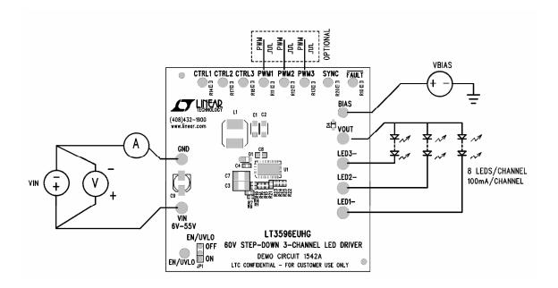
Figure 1. Proper Measurement Equipment Setup
