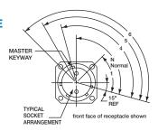
Note that insert arrangement does not rotate with master key/keyway
