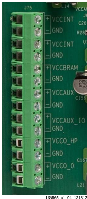
Figure 1-4: Core Power Terminal Block J75
