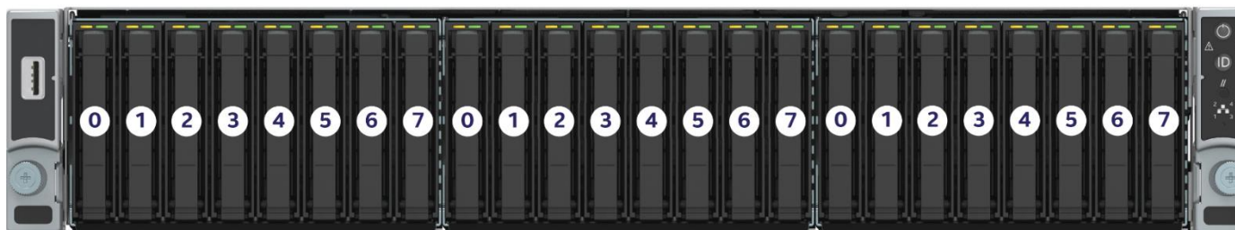
Figure 33. 2U 2.5" drive identification for each drive bay
