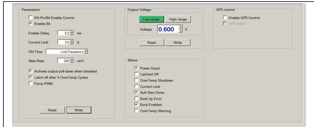
FIGURE 4-6: MIC23356 I 2 C Programmable Features Area – Low Range.
