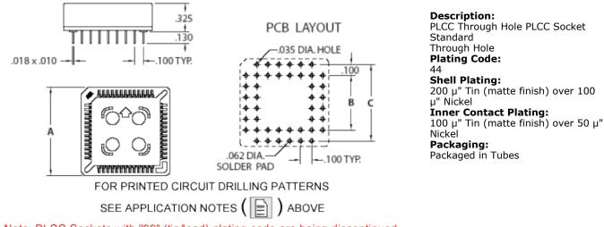
Note: PLCC Sockets with "99" (tin/lead) plating code are being discontinued and will only be available in RoHS compliant "44" (pure tin). "99" plating is still available in limited quantities until all existing stock is depleted.
