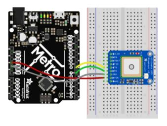
For an Arduino compatible, or any board that does not have an extra Hardware Serial port, we'll use Software Serial
