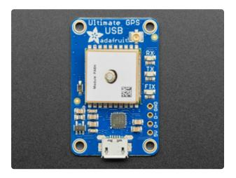
You can also skip the USB console cable, and just plug a Micro B cable directly from your computer to the Ultimate GPS USB
