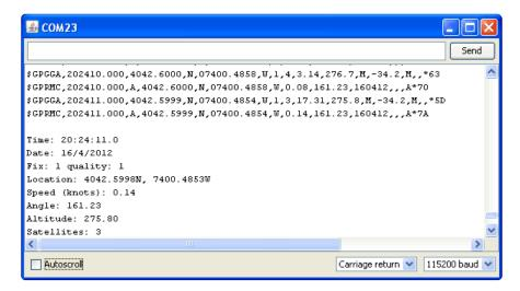
You'll only get correct time and location data if the GPS has a fix. Make sure it has an external antenna outside or is very close to a window and pointing up, to get GPS data! You'll usually get time information before location since you don't need as many satellites.
