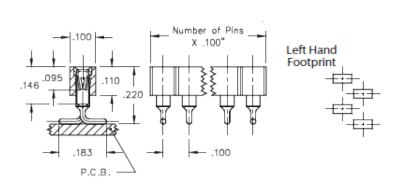
Interconnect Socket Surface Mount Socket Accepts .015"- .025" (0,38 - 0,635 mm) dia leads Single Row Surface Mount **Plating Code:** 43 Shell Plating: 200 µ" Tin (matte finish) over 100 µ" Nickel Inner Contact Plating:
