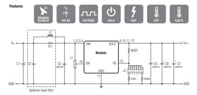
The additional aluminum electrolytic capacitor C1 is only for evaluation board protection purposes. It is mounted at the termination of the supply line and provides slight damping of possible oscillations of the series resonance circuit represented by the inductance of the supply line and the input capacitance. It is not essential for operation.
