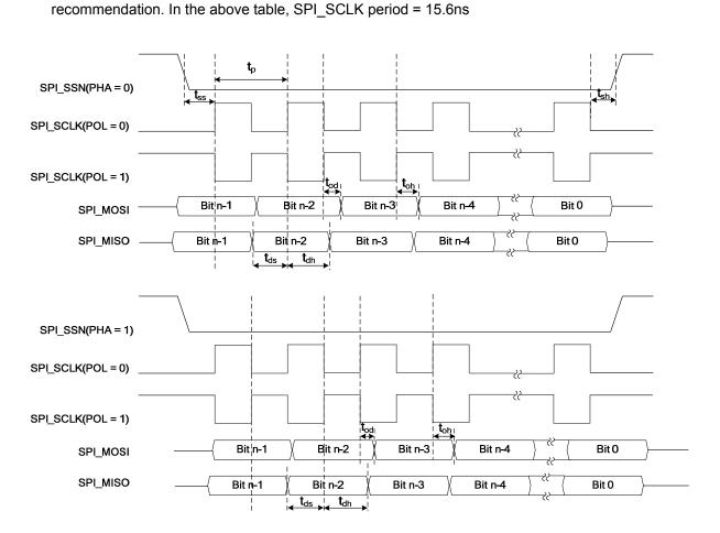
Figure 9-3 SPI Interface--Transmit and Receive in Master Mode
