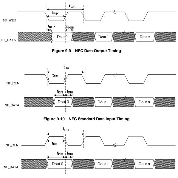
Figure 9-11 NFC EDO Data Input Timing
