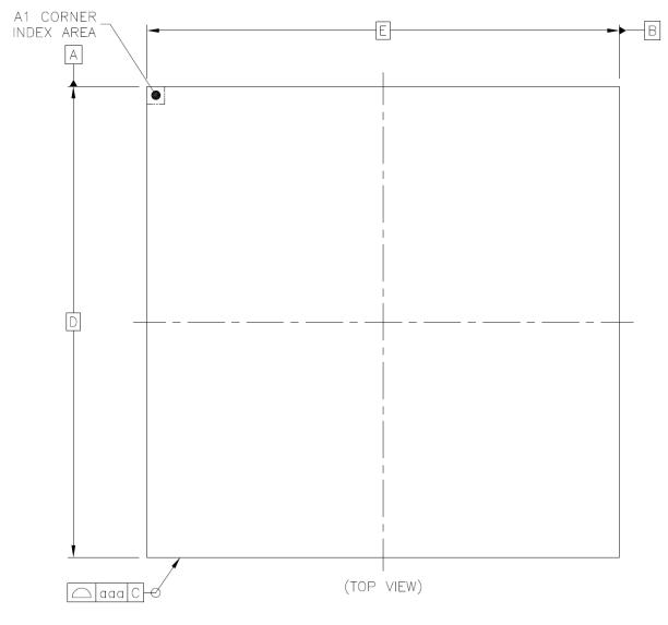
Figure3-5 Top View of 445BGA Package
