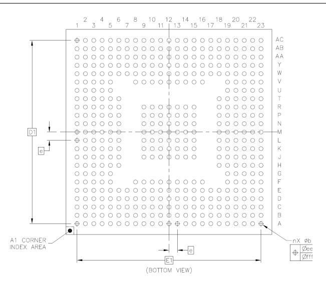
Figure 3-6 Bottom View of 445BGA Package
