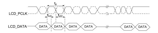
Figure 9-14 Data Output Timing for DPI Panel (falling edge capture)
