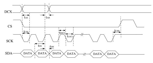
Figure 9-13 LCD Serial Interface Timing
