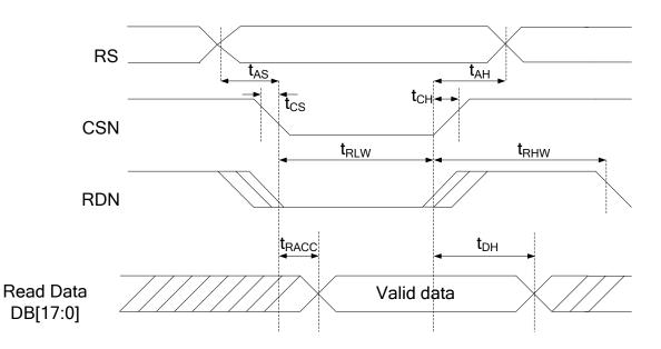
Figure 9-17 LCD Interface Timing for DBI Panel (Read Operation)
