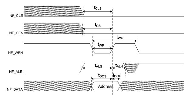
Figure 9-8 NFC Address Latch Timing
