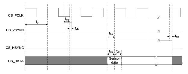
Figure 9-1 Sensor Interface Timing
