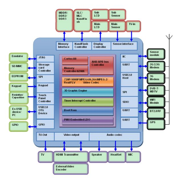
Figure 2-1 System Diagram of 445BGA
