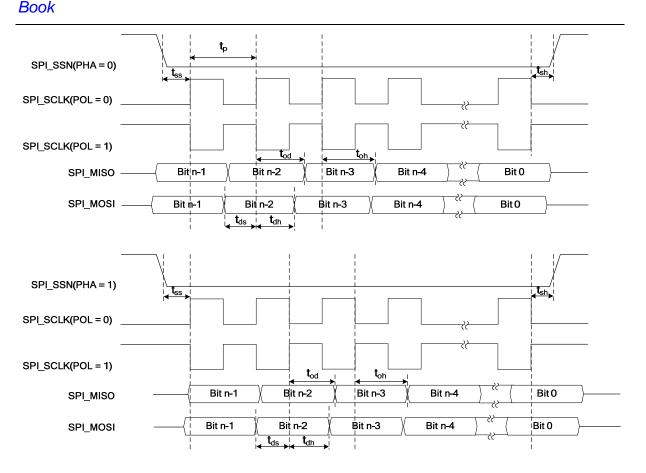
Figure 9-2 SPI Interface--Transmit and Receive in Slave Mode
