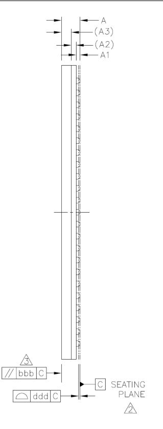
Figure 3-7 Side View of 445BGA Package
