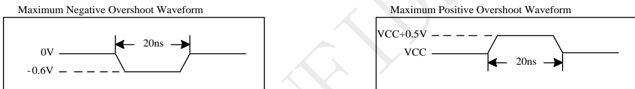
Figure 5-1 Maximum Overshoot Waveform
