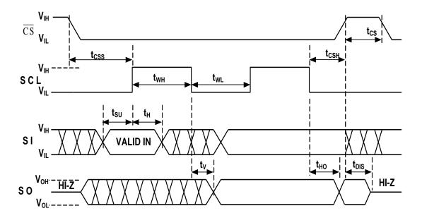
Figure 4: Synchronous Data Timing (for Mode 0)
