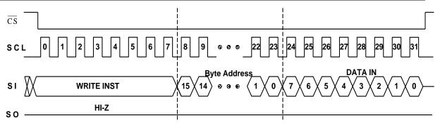
Figure 10: WRITE Timing
