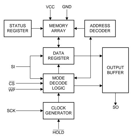
Figure 2: Block Diagram
