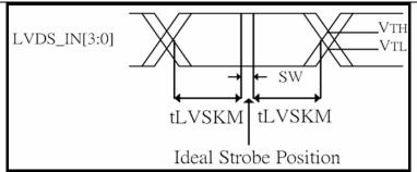
SW: Setup and Hold time Figure 5.1 Input signal data timing
