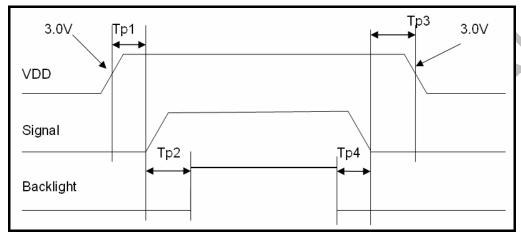
Figure 5.2 Interface power on/off sequenc
