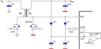
Figure 13. VAUX supply for CC regulation operation (from rectified SR MOSFET drain)
