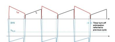
Figure 9. Timer anticipation for fixed frequency CCM operation (100 pF mounted on TON pin)
