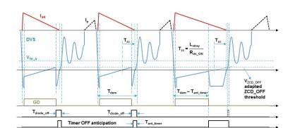
Figure 10. Timer anticipation for QR operating circuit (no capacitor mounted on TON pin)
