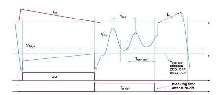
Figure 11. Blanking time after turn-off
