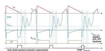
Figure 8. ZCD\_OFF threshold adapting for body diode target conduction
