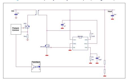
Figure 5. Fixed frequency CCM flyback adapter (CV regulation)
