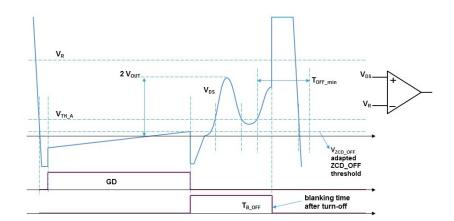
Figure 12. Comparator for blanking time termination
