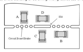
Stress strength according to he mounting position: A>B>C>D
