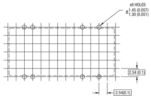
All dimensions in mm (inches)  $\pm 0.25(0.010)$ . All pins on a 2.54(0.10") pitch and within  $\pm 0.25(0.010)$  of true position.
