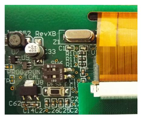
For normal operation the DIP switch remains in the default setting with switch 1 in the RUN position and switch 2 in the TCAL position. See figure above for the default settings.
