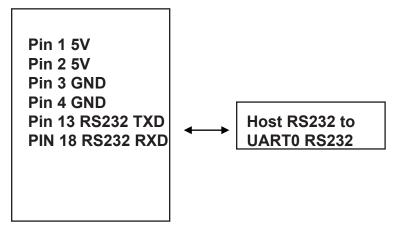
Note: If RS232 is not required, the MK-CY-043 can be hardware configured to utilize UART0 as another TTL-level UART in addition to UART1. Please contact our support department at support@amulettechnologies.com for details. For I/O requirements through SPI or I<sup>2</sup>C, also contact Amulet's support department
