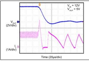
FIGURE 2-38: Short Circuit (MIC28512-1).
