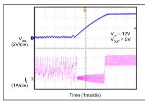
**FIGURE 2-39:** Output Recovery from Short Circuit to 2A.
