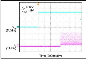
FIGURE 2-33: Start-Up Into Short Circuit (MIC28512-2).
