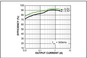
FIGURE 2-11: Efficiency ( $V_{IN} = 12V$ ) vs. Output Current (MIC28512-1).
