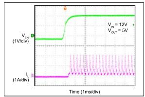
FIGURE 2-34: Enable into Short Circuit.
