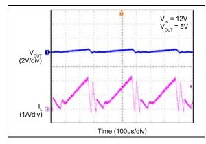
FIGURE 2-41: Short Circuit. (MIC28512-1)
