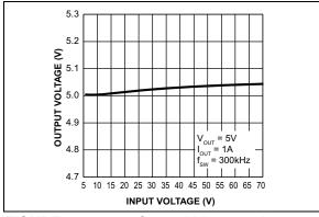
**FIGURE 2-7:** Output Voltage vs. Input Voltage.
