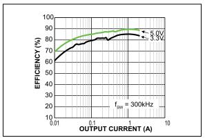
**FIGURE 2-12:** Efficiency  $(V_{IN} = 24V)$  vs. Output Current (MIC28512-1).
