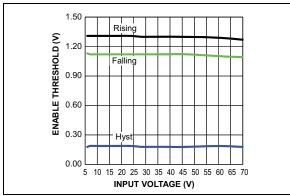
FIGURE 2-3: Enable Threshold vs. Input Voltage.
