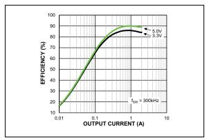
**FIGURE 2-18:** Efficiency  $(V_{IN} = 24V)$  vs. Output Current (MIC28512-2).
