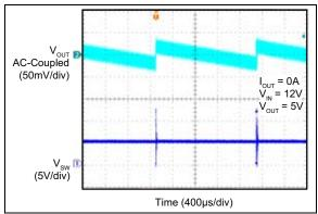
**FIGURE 2-49:** MIC28512-1 Switching Waveform ( $I_{OUT} = 0A$ ).
