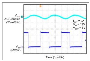
**FIGURE 2-50:** MIC28512-2 Switching Waveform ( $I_{OUT} = 0A$ ).
