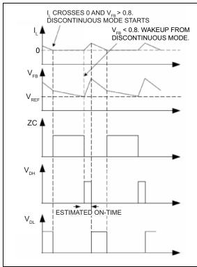
FIGURE 4-4: MIC28512-1 Control Loop Timing (Discontinuous Mode).
