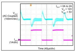
**FIGURE 2-54:** MIC28512-2 Load Transient Response (0A to 2A).
