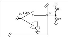
FIGURE 5-1: Voltage Divider Configuration.
