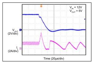
FIGURE 2-36: Short Circuit (MIC28512-2).
