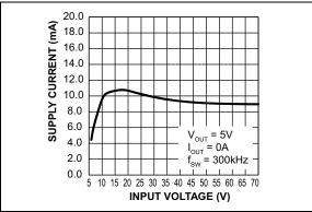
**FIGURE 2-14:** V<sub>IN</sub> Operating Supply Current vs. Input Voltage (MIC28512-2).
