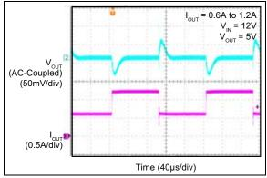
**FIGURE 2-55:** MIC28512-1 Load Transient Response (0A to 0.6A).
