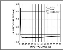
**FIGURE 2-1:** V<sub>IN</sub> Operating Supply Current vs. Input Voltage (MIC28512-1).
