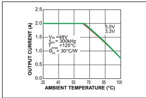
FIGURE 2-25: 48V Input Thermal Derating.
