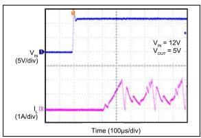
**FIGURE 2-42:** Input Voltage Applied with Output Shorted (MIC28512-1).
