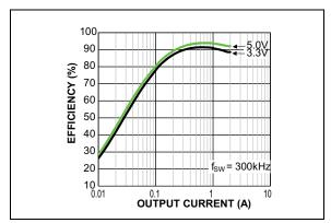
**FIGURE 2-17:** Efficiency  $(V_{IN} = 12V)$  vs. Output Current (MIC28512-2).
