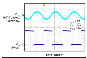
**FIGURE 2-51:** MIC28512-1 Switching Waveform ( $I_{OUT} = 2A$ ).
