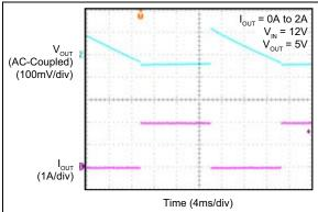
FIGURE 2-53: MIC28512-1 Load Transient Response (0A to 2A).
