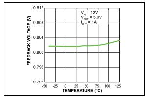
**FIGURE 2-6:** Feedback Voltage vs. Temperature (MIC28512-1).
