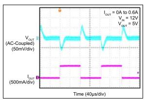
**FIGURE 2-56:** MIC28512-2 Load Transient Response (0A to 0.6A).
