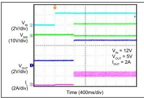
**FIGURE 2-31:** V<sub>IN</sub> Start-Up with 1V Pre-Biased Output (MIC28512-2).
