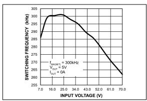
**FIGURE 2-26:** Switching Frequency vs. Input Voltage (MIC28512-2).
