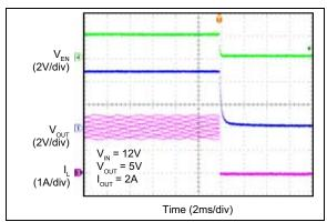
**FIGURE 2-30:** Enable Turn-Off Delay and Fall Time (MIC28512-2).
