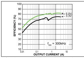
**FIGURE 2-13:** Efficiency  $(V_{IN} = 48V)$  vs. Output Current (MIC28512-1).
