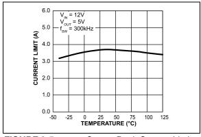
**FIGURE 2-5:** Output Peak Current Limit vs. Temperature.
