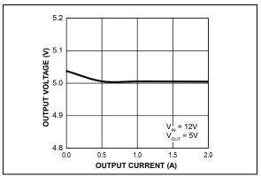
**FIGURE 2-10:** Output Voltage vs. Output Current (MIC28512-1).
