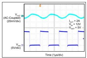
**FIGURE 2-52:** MIC28512-2 Switching Waveform ( $I_{OUT} = 2A$ ).
