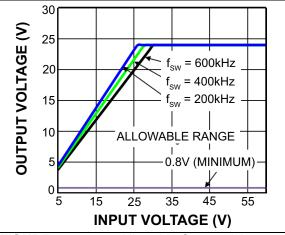
FIGURE 4-1: Allowable Output Voltage Range vs. Input Voltage.
