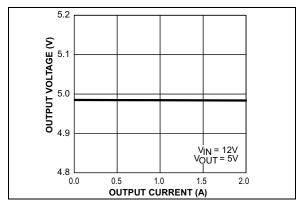
FIGURE 2-16: Output Voltage vs. Output Current (MIC28512-2).
