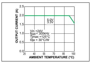
FIGURE 2-24: 24V Input Thermal Derating.
