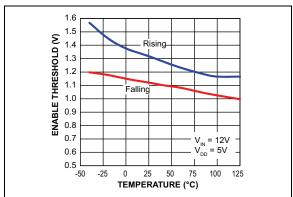
FIGURE 2-8: Enable Threshold vs. Temperature.
