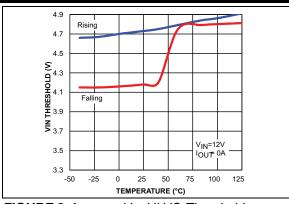
**FIGURE 2-4:** V<sub>IN</sub> ULVO Threshold vs. Temperature.
