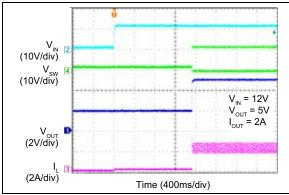
**FIGURE 2-32:** V<sub>IN</sub> Start-Up with 2V Pre-Biased Output (MIC28512-2).
