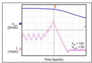
FIGURE 2-35: Inductor Peak Current (Output Short Applied) (MIC28512-2).
