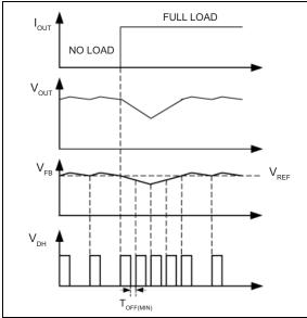
FIGURE 4-3: MIC28512 Load Transient Response.
