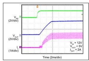
FIGURE 2-29: Enable Turn-On Delay and Rise Time (MIC28512-2).
