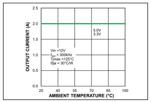
FIGURE 2-23: 12V Input Thermal Derating.
