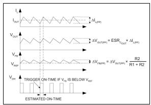
FIGURE 4-2: MIC28512 Control Loop Timing.
