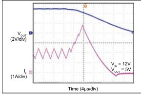
FIGURE 2-37: Inductor Peak Current (Output Short Applied) (MIC28512-1).
