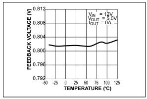
**FIGURE 2-15:** Feedback Voltage vs. Temperature (MIC28512-2).
