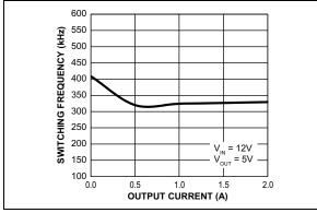
**FIGURE 2-9:** Switching Frequency vs. Output Current (MIC28512-2).
