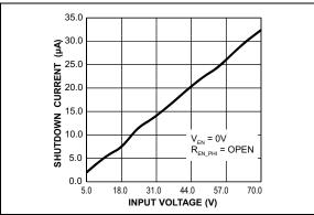
**FIGURE 2-2:** V<sub>IN</sub> Shutdown Current vs. Input Voltage.
