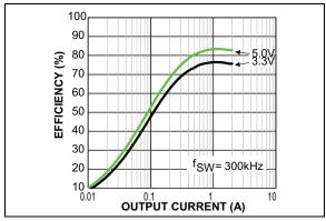
**FIGURE 2-19:** Efficiency  $(V_{IN} = 48V)$  vs. Output Current (MIC28512-2).
