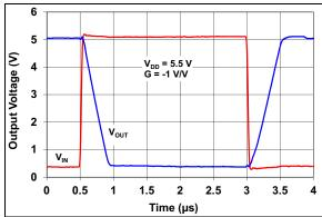
FIGURE 2-45: Inverting Large Signal Step Response.
