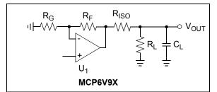
FIGURE 4-9: Output Load.
