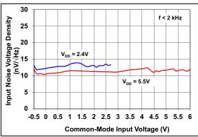
**FIGURE 2-35:** Input Noise Voltage Density vs. Input Common-Mode Voltage.
