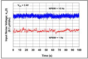
**FIGURE 2-38:** Input Noise vs. Time with 1 Hz and 10 Hz Filters and  $V_{DD} = 2.4V$ .
