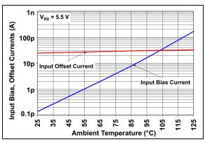
**FIGURE 2-14:** Input Bias and Offset Currents vs. Ambient Temperature with  $V_{DD} = 5.5V$ .
