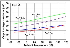
**FIGURE 2-18:** Output Voltage Headroom vs. Ambient Temperature.
