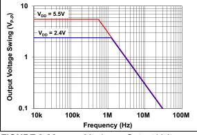
FIGURE 2-30: Maximum Output Voltage Swing vs. Frequency.
