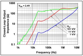
**FIGURE 2-28:** Closed-Loop Output Impedance vs. Frequency with  $V_{DD} = 2.2V$ .
