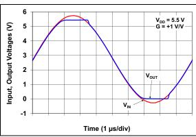
FIGURE 2-41: The MCP6V96/6U/7/9 Family Shows No Input Phase Reversal with Overdrive.
