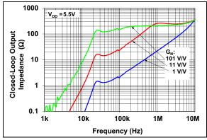
**FIGURE 2-29:** Closed-Loop Output Impedance vs. Frequency with  $V_{DD} = 5.5V$ .
