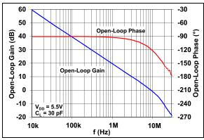
**FIGURE 2-24:** Open-Loop Gain vs. Frequency with  $V_{DD} = 5.5V$ .
