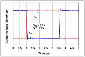
FIGURE 2-44: Inverting Small Signal Step Response.
