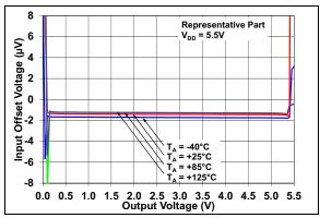
**FIGURE 2-7:** Input Offset Voltage vs. Output Voltage with  $V_{DD} = 5.5V$ .
