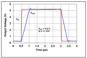
FIGURE 2-43: Noninverting Large Signal Step Response.
