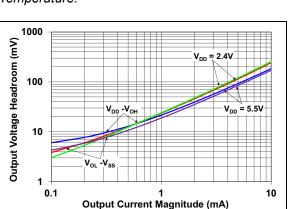
FIGURE 2-17: Output Voltage Headroom vs. Output Current.
