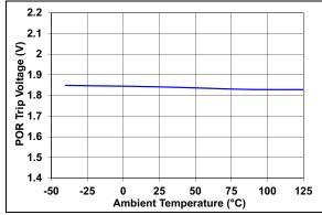
**FIGURE 2-21:** Power-On Reset Voltage vs. Ambient Temperature.
