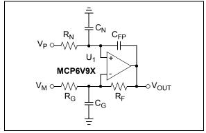
FIGURE 4-10: Amplifier with Parasitic Capacitance.
