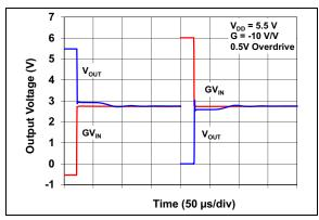
**FIGURE 2-47:** Output Overdrive Recovery vs. Time with G = -10 V/V.
