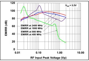
FIGURE 2-32: EMIRR vs. Input Voltage.
