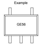
5-Lead SOT-23 (MCP6V96, MCP6V96U)
