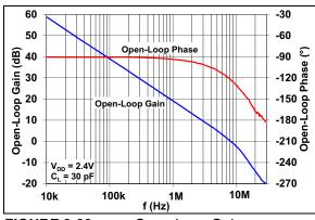
**FIGURE 2-23:** Open-Loop Gain vs. Frequency with  $V_{DD} = 2.4V$ .
