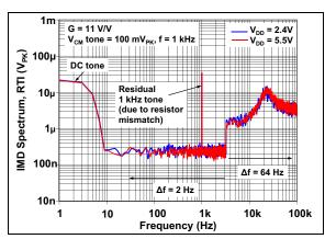
**FIGURE 2-36:** Intermodulation Distortion vs. Frequency with V<sub>CM</sub> Disturbance (see Figure 1-6).
