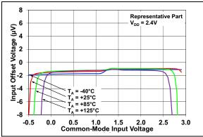
**FIGURE 2-8:** Input Offset Voltage vs. Common-Mode Voltage with  $V_{DD} = 2.4V$ .
