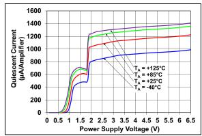
FIGURE 2-20: Supply Current vs. Power Supply Voltage.
