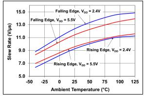
FIGURE 2-46: Slew Rate vs. Ambient Temperature.
