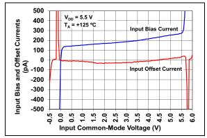
**FIGURE 2-13:** Input Bias and Offset Currents vs. Common-Mode Input Voltage with  $T_A = +125$ °C.
