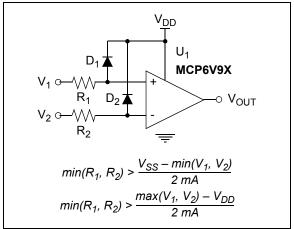
FIGURE 4-6: Protecting the Analog Inputs Against High Currents.
