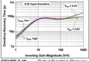
**FIGURE 2-48:** Output Overdrive Recovery Time vs. Inverting Gain.
