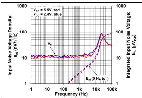
FIGURE 2-34: Input Noise Voltage Density and Integrated Input Noise Voltage vs. Frequency.
