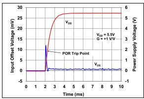
**FIGURE 2-40:** Input Offset Voltage vs. Time at Power-Up.
