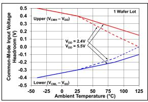
**FIGURE 2-16:** Input Common-Mode Voltage Headroom (Range) vs. Ambient Temperature.
