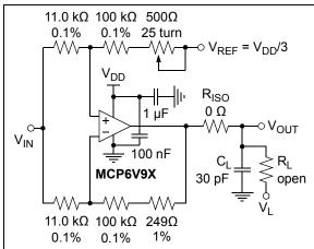
FIGURE 1-6: Test Circuit for Dynamic Input Behavior.
