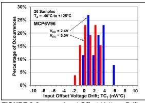
FIGURE 2-2: Input Offset Voltage Drift.
