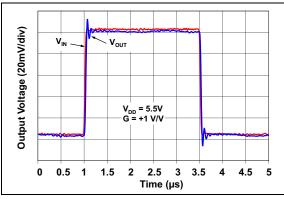
FIGURE 2-42: Noninverting Small Signal Step Response.
