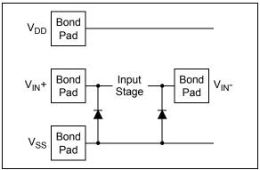
FIGURE 4-4: Simplified Analog Input ESD Structures.
