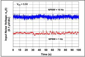
**FIGURE 2-39:** Input Noise vs. Time with 1 Hz and 10 Hz Filters and  $V_{DD} = 5.5V$ .
