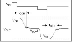
FIGURE 1-3: Output Overdrive Recovery.
