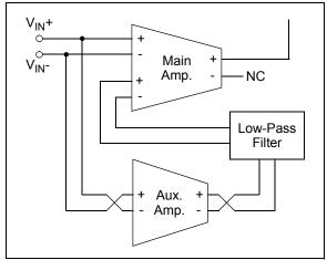
FIGURE 4-3: Second Chopping Clock Phase; Equivalent Amplifier Diagram.
