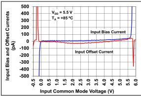
**FIGURE 2-12:** Input Bias and Offset Currents vs. Common-Mode Input Voltage with  $T_A = +85$ °C.
