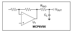
**FIGURE 4-7:** Output Resistor, R<sub>ISO</sub>, Stabilizes Capacitive Loads.
