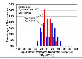
FIGURE 2-3: Input Offset Voltage Quadratic Temperature Coefficient.
