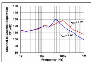
**FIGURE 2-33:** Channel-to-Channel Separation vs. Frequency.
