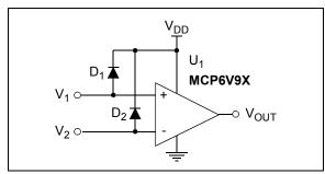
**FIGURE 4-5:** Protecting the Analog Inputs Against High Voltages.
