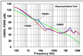
FIGURE 2-22: CMRR and PSRR vs. Frequency.
