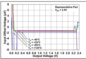
**FIGURE 2-6:** Input Offset Voltage vs. Output Voltage with  $V_{DD} = 2.4V$ .
