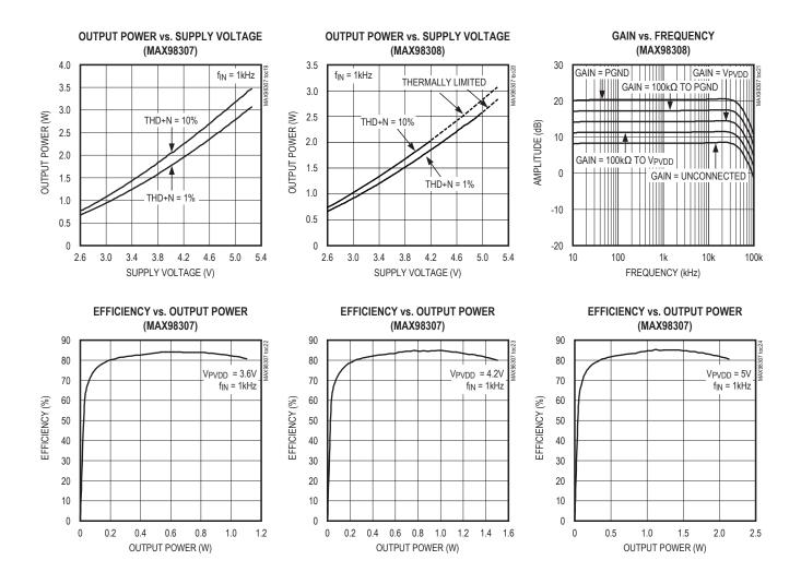
$(V_{PVDD} = V_{CC} = V_{\overline{SHDN}} = 3.6V, V_{PGND} = V_{GND} = 0V, Z_{L} = 8\Omega + 68\mu \text{H between OUT+ and OUT-, } A_{V} = 14.5 \text{dB (MAX98307 R}_{\text{IN+}} = R_{\text{IN-}} = 10 \text{k}\Omega, R_{\text{FB+}} = R_{\text{FB-}} = 20 \text{k}\Omega), C_{\text{IN+}} = C_{\text{IN-}} = 0.33 \mu \text{F, AC measurement bandwidth 20Hz to 20kHz.)}$
