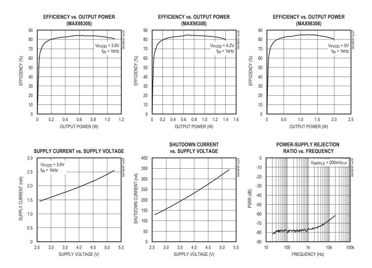
$(V_{PVDD} = V_{CC} = V_{\overline{SHDN}} = 3.6V, V_{PGND} = V_{GND} = 0V, Z_L = 8\Omega + 68\mu\text{H between OUT+ and OUT-, } A_V = 14.5dB \text{ (MAX98307 R}_{\text{IN+}} = R_{\text{IN-}} = 10k\Omega, R_{\text{FB+}} = R_{\text{FB-}} = 20k\Omega), C_{\text{IN+}} = C_{\text{IN-}} = 0.33\mu\text{F, AC measurement bandwidth 20Hz to 20kHz.)}$
