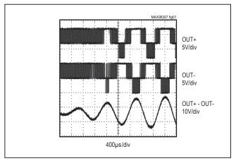
Figure 1. Class DG Multilevel Operation
