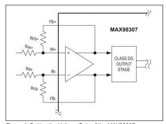
Figure 4. Setting the Voltage Gain of the MAX98307
