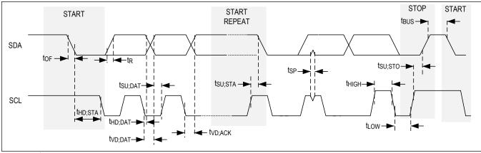
Figure 1. I<sup>2</sup>C Timing Diagram
