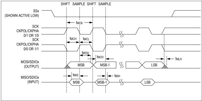
Figure 2. SPI Master Mode Timing Diagram
