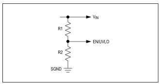
Figure 2. Setting the Input Undervoltage Lockout
