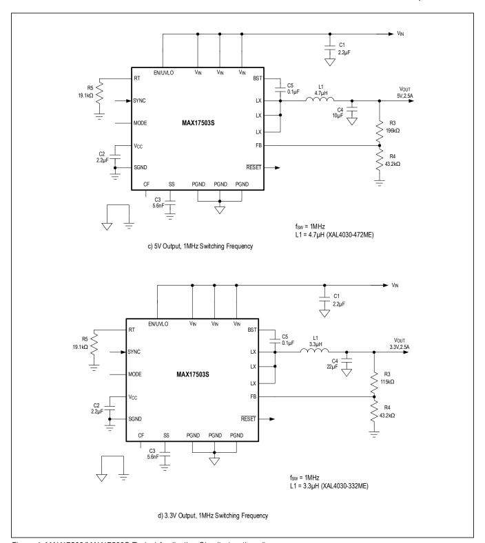
Figure 4. MAX17503/MAX17503S Typical Application Circuits (continued)
