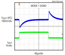
MAX17503 3.3V OUTPUT, PWM MODE (LOAD CURRENT STEPPED FROM 1A TO 2A), FIGURE 4b CIRCUIT
