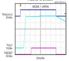
MAX17503 SOFT-START/SHUTDOWN FROM EN/UVLO, 3.3V OUTPUT, PFM MODE, 5mA LOAD CURRENT, FIGURE 4b CIRCUIT
