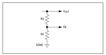
Figure 3. Setting the Output Voltage
