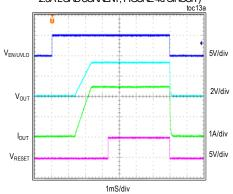
MAX17503S, SOFT-START/SHUTDOWN FROMENUMLO, 5V OUTPUT, PFM MODE 5MA LOAD CURRENT, FIGURE 4c CIRCUIT)
