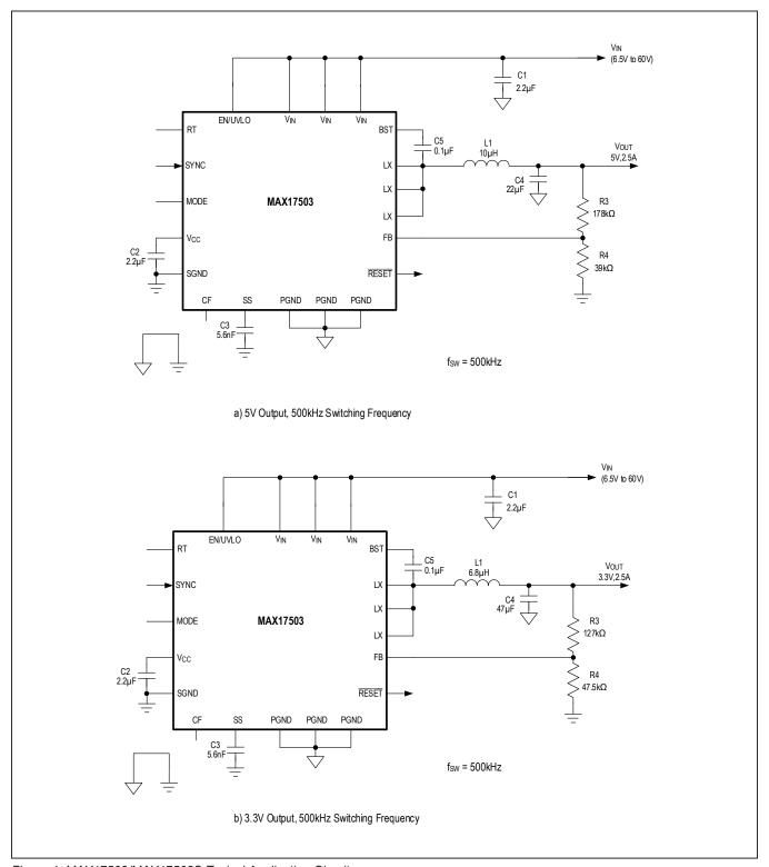
Figure 4. MAX17503/MAX17503S Typical Application Circuits
