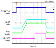
MAX17503 SOFT-START/SHUTDOWN FROM EN/UVL 5V OUTPUT, PFM MODE, 5mA LOAD CURRENT, FIGURE 4a CIRCUIT
