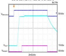
MAX17503S, SOFT-START/SHUTDOWN FROMENUMLO, 3.3V OUTPUT, PFMMODE 5MA LOAD CURRENT, FIGURE 4d CIRCUIT)
