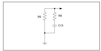
Figure 1. Setting the Switching Frequency
