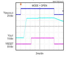
MAX17503S, SOFT-START/ SHUTDOWNFROM ENUMLO, 3.3V OUTPUT, 2.5A LOAD CURRENT, FIGURE 4d CIRCUIT)
