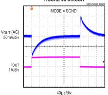
MAX17503 5V OUTPUT, PWM MODE (LOAD CURRENT STEPPED FROM NO-LOAD TO 1A),
