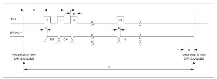
Figure 1. Timing Diagram for Data Read After Conversion
