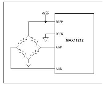
Figure 7. Resistive Bridge Measurement Circuit
