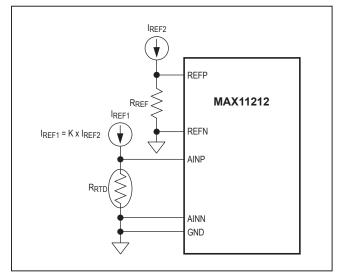
Figure 6. RTD Temperature Measurement Circuit
