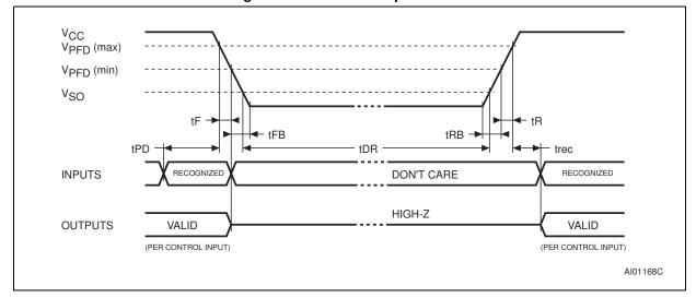
Figure 8. Power down/up mode AC waveforms
