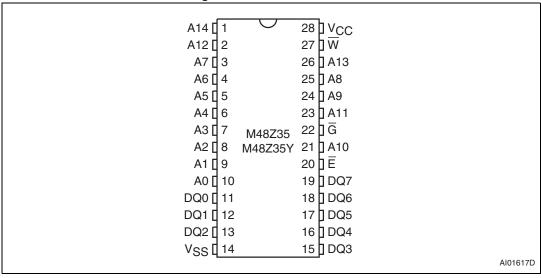
Figure 3. SOIC connections
