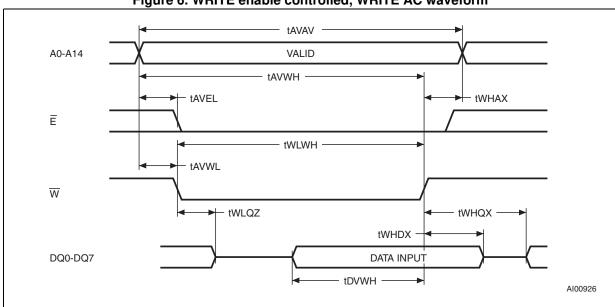
Figure 6. WRITE enable controlled, WRITE AC waveform
