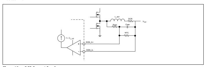
Figure 15 **DCR Current Sensing**
