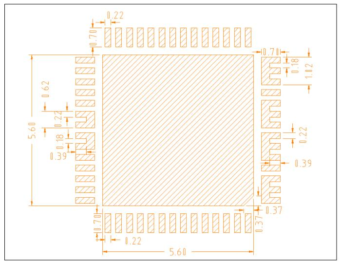
Figure 39 PCB PAD Size
