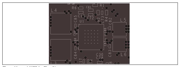
Figure 22 LAYER 3 – Signal Layer
