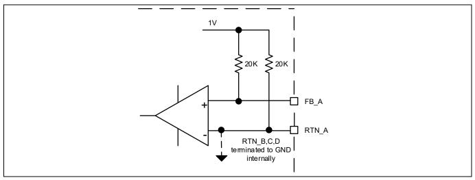
Figure 12 Output Voltage Sensing impedance
