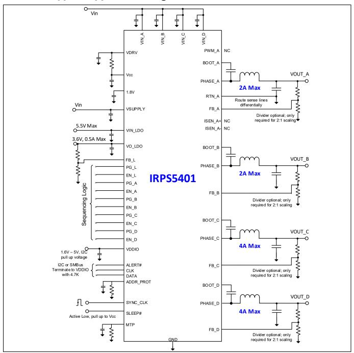
IRPS5401 in 5 output configuration with Vcc from internal LDO Figure 5
