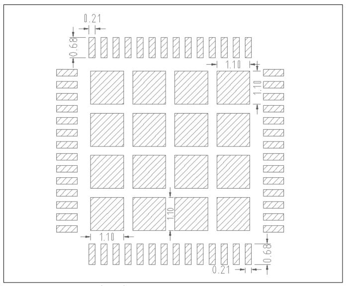
Figure 41 Solder paste stencil pad size
