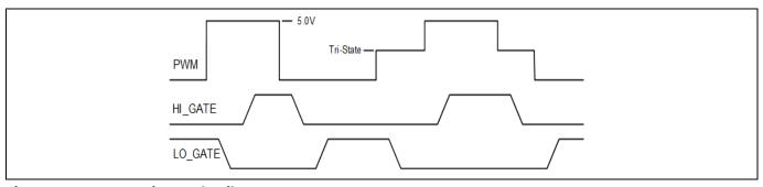
Figure 10 PWM\_A tri-state details
