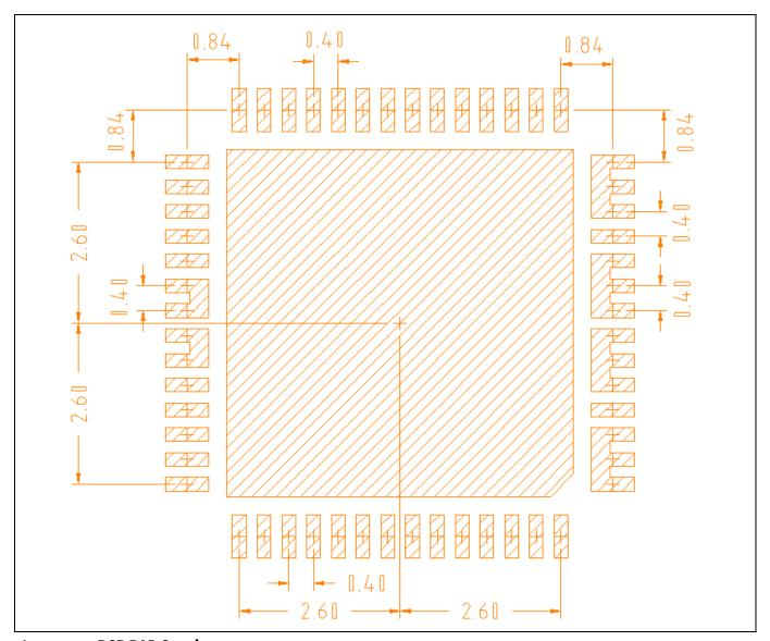
Figure 40 PCB PAD Spacing
