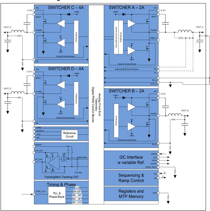
Figure 4 **IRPS5401 Block Diagram**
