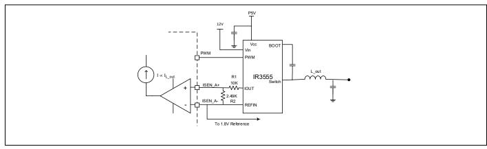
Figure 16 Rdson Current Sensing
