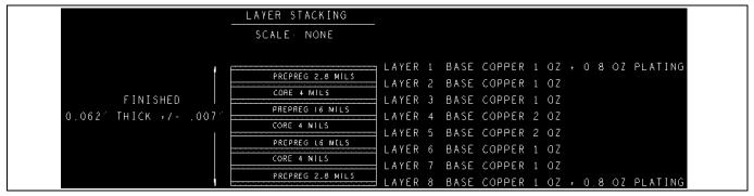
Figure 36 PCB construction details (8 layers, 11.6 oz total Cu Thickness)
