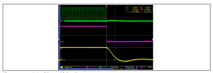
Figure 14 OVP with vpu\_high\_release\_en=0
