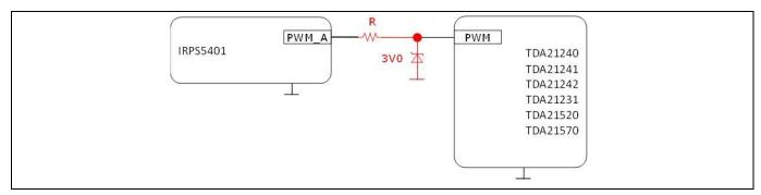
Figure 11 Zener clamp details when using power stages that only support 3.3V PWM input
