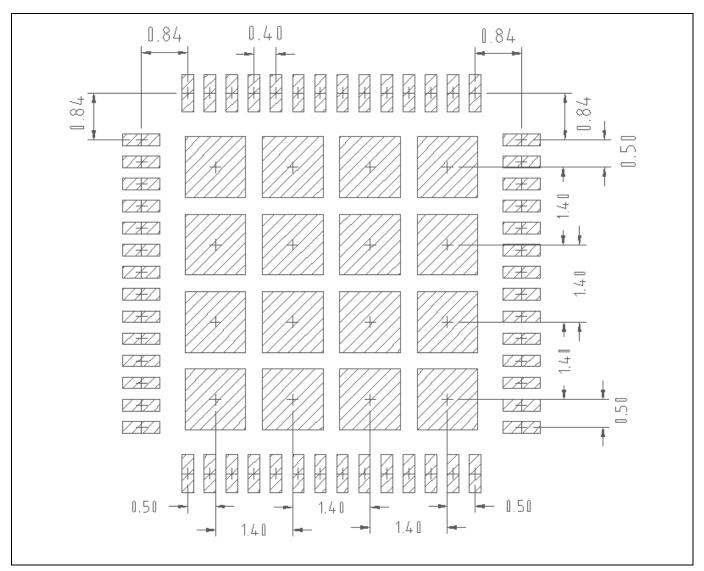
Figure 42 Solder paste stencil pad spacing
