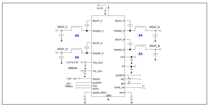
Figure 1 **IRPS5401 Basic application circuit**
