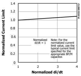
Figure 27. Standard Current Limit vs. di/dt.
