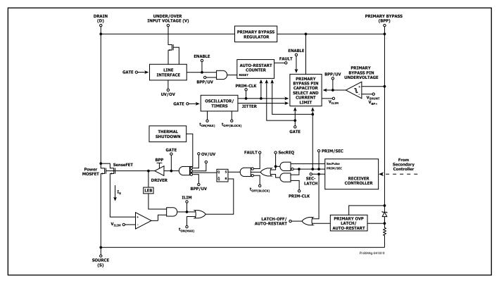
Figure 3. Primary Controller Block Diagram.
