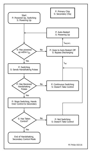
Figure 7. Primary-Secondary Handshake Flowchart.
