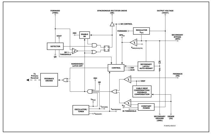
Figure 4. Secondary Controller Block Diagram.
