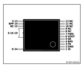
Figure 5. Pin Configuration.
