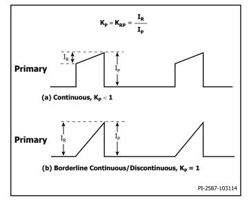
Figure 19. Continuous Conduction Mode Current Waveform, KP < 1.
