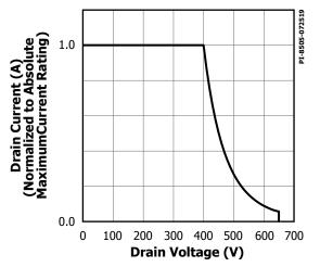
Figure 21. Maximum Allowable Drain Current vs. Drain Voltage.
