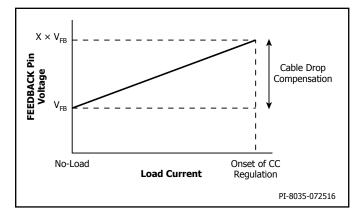
Figure 8. Cable Drop Compensation Characteristics.
