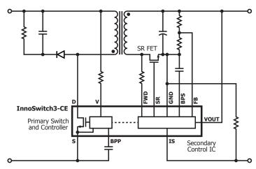
Figure 1. Typical Application schematic.
