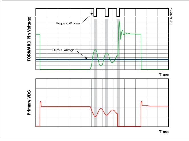
Figure 9. Intelligent Quasi-Resonant Mode Switching.
