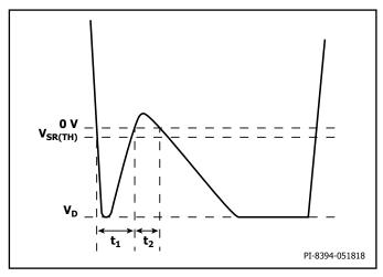
Figure 14. Unacceptable FORWARD Pin Waveform before Handshake with Body Diode Conduction During Flyback Cycle. Note:
