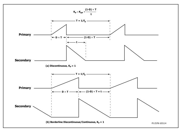
Figure 20. Discontinuous Conduction Mode Current Waveform,  $K_p > 1$ .
