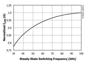
Figure 6. Normalized Primary Current vs. Frequency.
