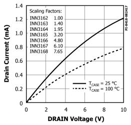
Figure 22. Output Characteristics.
