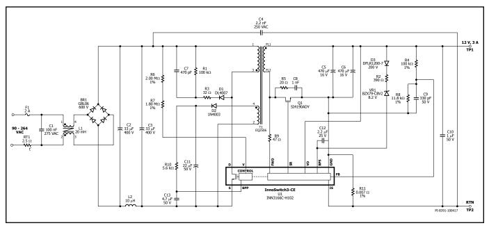
Figure 11. 12 V, 3 A Charger/Adapter.
