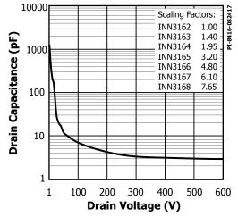
Figure 23. C<sub>oss</sub> vs. Drain Voltage.
