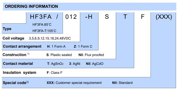
Notes: 1) We recommend flux proofed types for a clean environment (free from contaminations like H2S, SO2, NO2, dust, etc.). We suggest to choose plastic sealed types and validate it in real application for an unclean environment (with contaminations like H<sub>2</sub>S, SO<sub>2</sub>, NO<sub>2</sub>, dust, etc).
