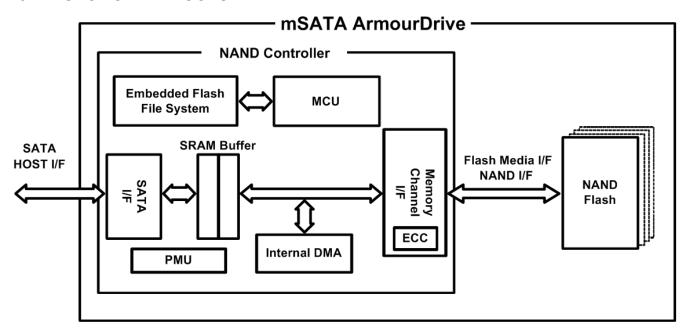
Figure 2-1: mSATA ArmourDrive Block Diagram
