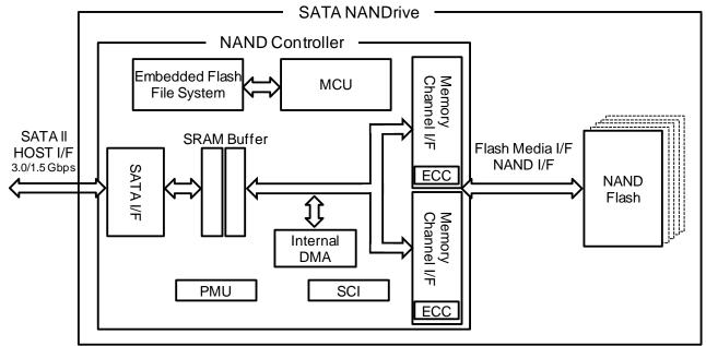
Figure 2-1: SATA NANDrive Block Diagram
