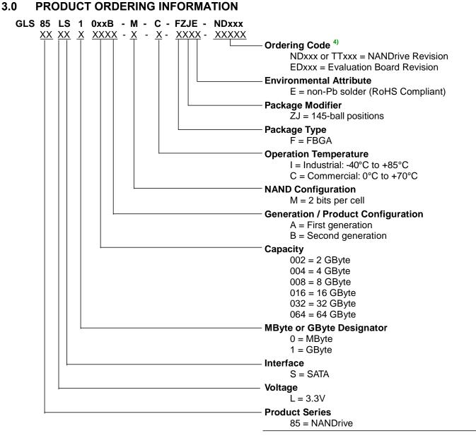
4) Note that the top side marking on the package typically does not include ordering codes (e.g. NDxxx), unless it is a special C-SPEC (custom specification) which is required by the end-customer to be marked on the device.
