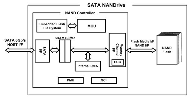
Figure 2-1: SATA NANDrive Block Diagram
