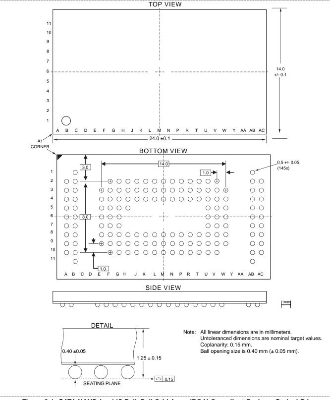
Figure 3-1: SATA NANDrive 145-Ball, Ball Grid Array (BGA) Greenliant Package Code: LBJ
