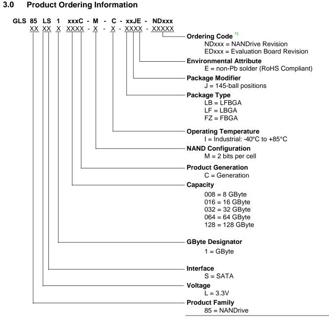
1) Note that the top side marking on the package typically does not include ordering codes (e.g. NDxxx), unless it is a special C-SPEC (custom specification) which is required by the end-customer to be marked on the device.
