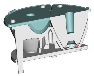
Figure 2: Cross-section view of the assembly shows the lenses touching the PCB. The assembly holder provides proper alignment between the lenses and the LEDs.
