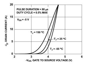
Figure 5. Transfer Characteristics
