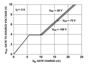
Figure 7. Gate Charge Characteristics
