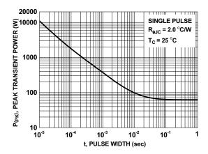
Figure 12. Single Pulse Maximum Power Dissipation
