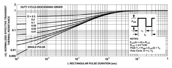
Figure 13. Junction-to-Case Transient Thermal Response Curve
