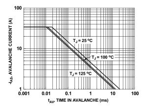
Figure 9. Unclamped Inductive Switching Capability
