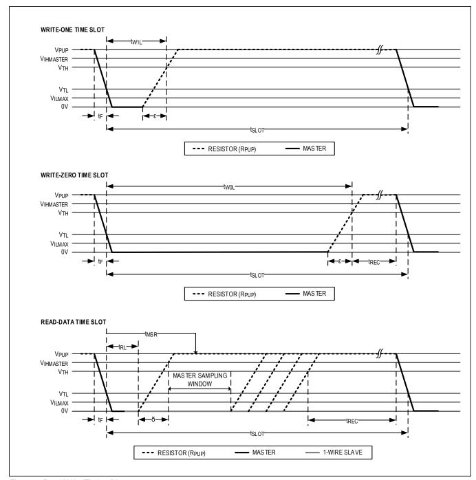
Figure 4. Read/Write Timing Diagrams
