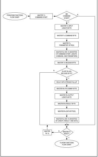
Figure 1. Device Function Flow Chart
