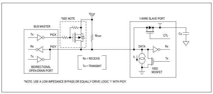
Figure 2. Hardware Configuration
