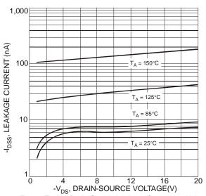
Fig. 10 Typical Drain-Source Leakage Current vs. Voltage
