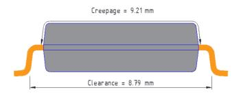
Figure 45. The Creepage and Clearance for the CT431's SOICW-16 package
