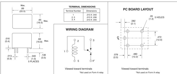
Dimensions in inches with metric equivalents in parentheses. Tolerance: ±0.010"
