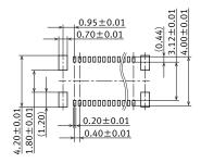
Recommended metal mask pattern Metal mask thickness: When 120 μm (Terminal opening ratio: 60%) (Metal-part opening ratio: 100%)
