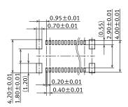
■ Keep the PC board warp no more than 0.03 mm in relation to the overall length of the connector.
