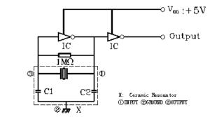
X: Ceramic Resonator C1=C2: 15pF ±20% 1: INPUT 2: GROUND 3: OUTPUT
